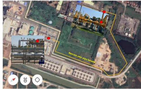
Gambar 5. Ilustrasi Jalur pipa Jumperline FCV Jawa 1 – SKG Cilamaya
