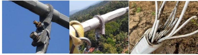
Figure 16. Melted Transmission Component
